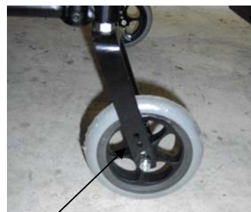
Diagram #18 Caster fork positions
