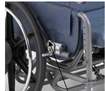
Wheel lock in unlocked position. (Pull toward front of chair to lock)
